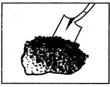
**APPLY:** Shovel or pour UPM<sup>®</sup> mix into the hole. Level out 25% higher than the existing pavement to allow for compaction. If patch is deeper than 4", apply and compact in separate 2" layers. Apply only over a solid base.
